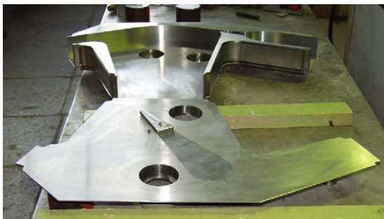
Fig. 5. Main elements of lithium mock-up.
